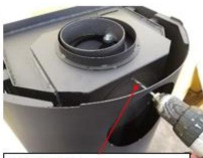
drilling of riverts
