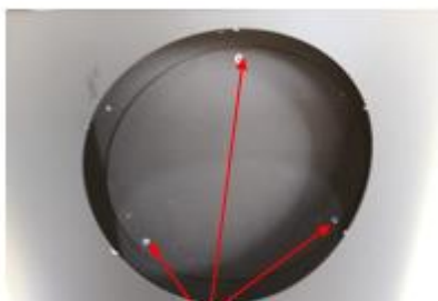
drilling with tool dia. 8mm
