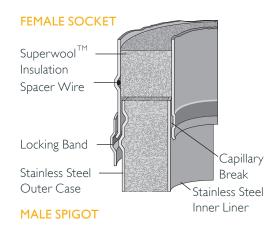
Sleeve joint with locking band for:
