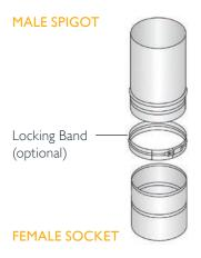
Sleeve joint with optional locking band for:
